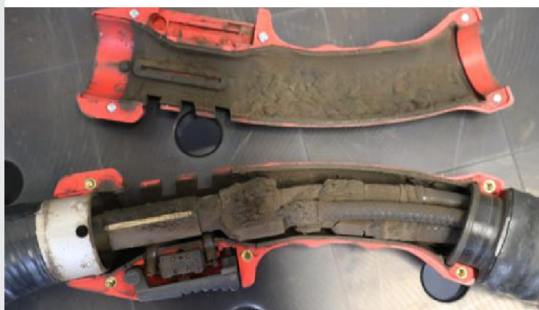
Conventional fume extraction torch
